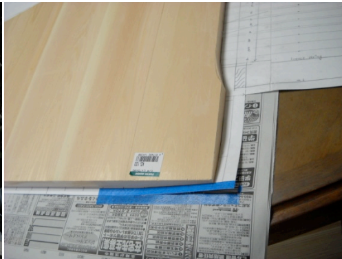
You should enough be careful that there is a enough space ,say 2mm, between the keyboard blank the rack
