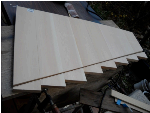
You should enough be careful that there is a enough space ,say 2mm, between the keyboard blank the rack
