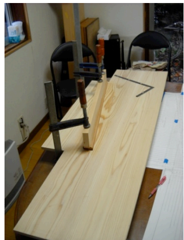
The balance rail is glued to the bottom. You have to pay enough attention to the position of the balance rail
