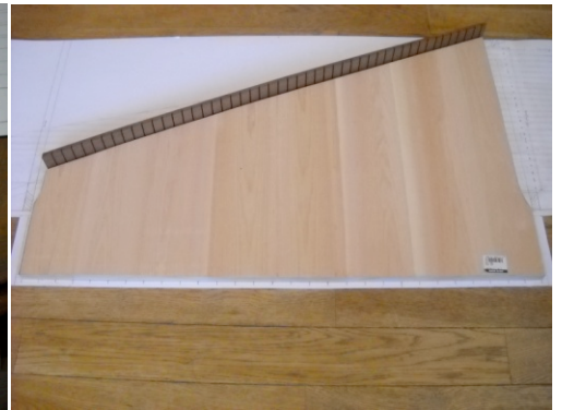
You should enough be careful that there is a enough space ,say 2mm, between the keyboard blank the rack
