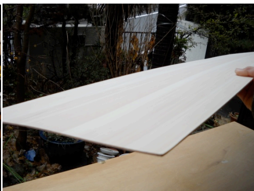
The middle photo above shows that the sound board may be too stiff. You may know where it will be too stiff under the sun. I use very good Japanese cypress for the soundboard. I make it 1.8mm thick at the treble around 2.2 the thickest.
