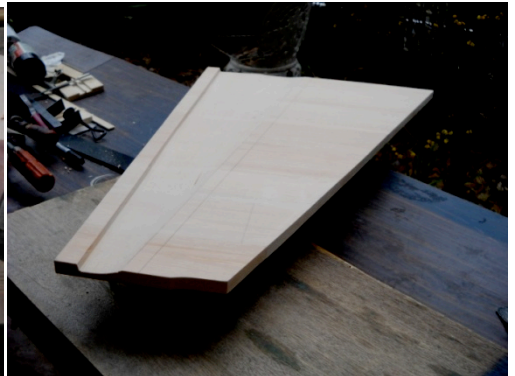
You should enough be careful that there is a enough space ,say 2mm, between the keyboard blank the rack
