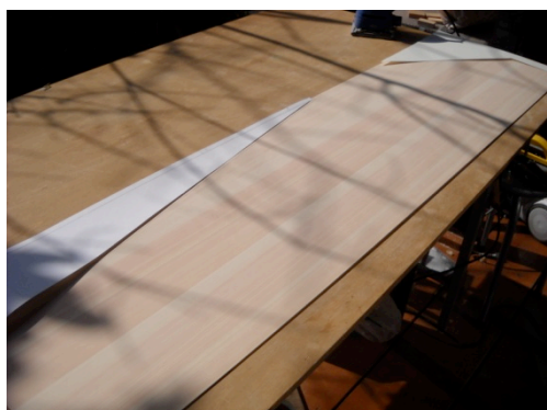
The middle photo above shows that the sound board may be too stiff. You may know where it will be too stiff under the sun. I use very good Japanese cypress for the soundboard. I make it 1.8mm thick at the treble around 2.2 the thickest.
