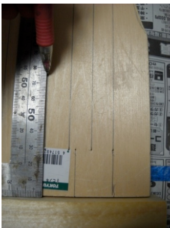
The balance rail is glued to the bottom. You have to pay enough attention to the position of the balance rail
