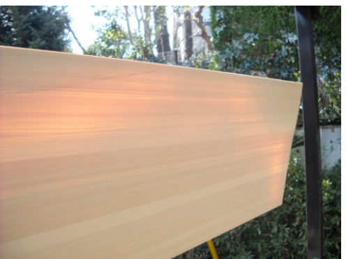
The middle photo above shows that the sound board may be too stiff. You may know where it will be too stiff under the sun. I use very good Japanese cypress for the soundboard. I make it 1.8mm thick at the treble around 2.2 the thickest.
