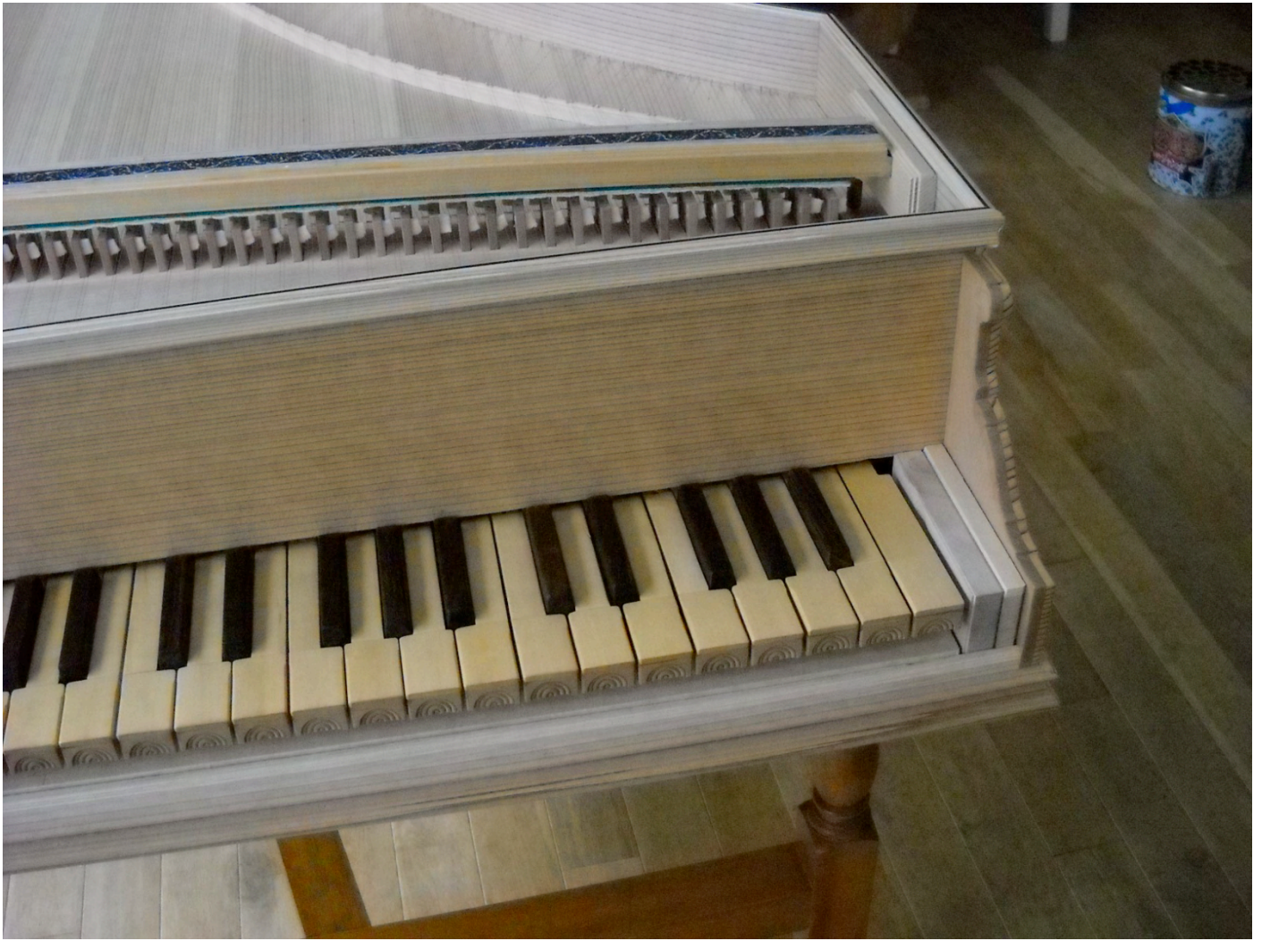
The key blocks at both end of the keyboard and a block for semitone transposing are made from hard wood though the key blocks are not glued yet.
