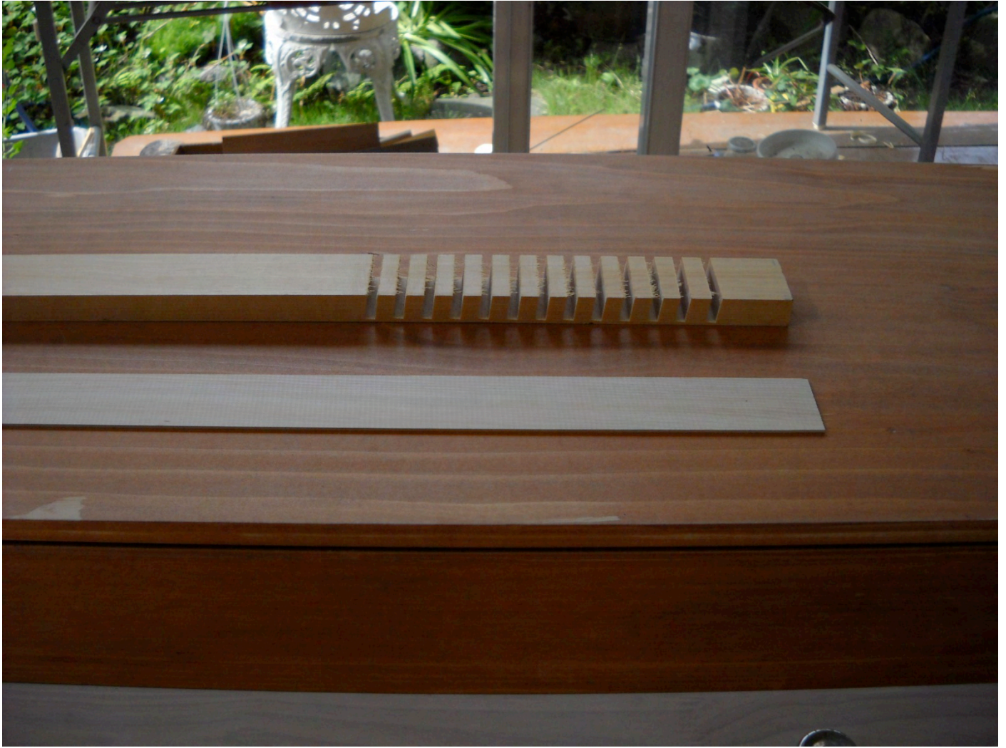
This photo is to show how the box slide is made. The mortises are cut angled because the back side of the wrest plank is angled. The veneer wood is glued to complete the mortises for the jacks.
