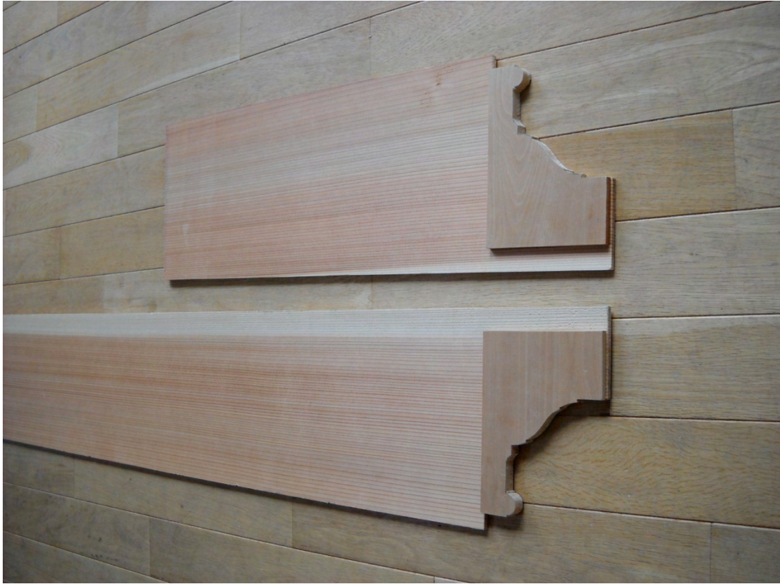
The fronts of spine and the cheek are now trimmed accurately to the pattern.
