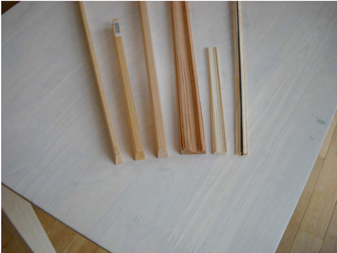
The three at the left are the bars of the sound board, the three at the right are the moldings, bottom molding, top side molding and the cap molding (left to right).
