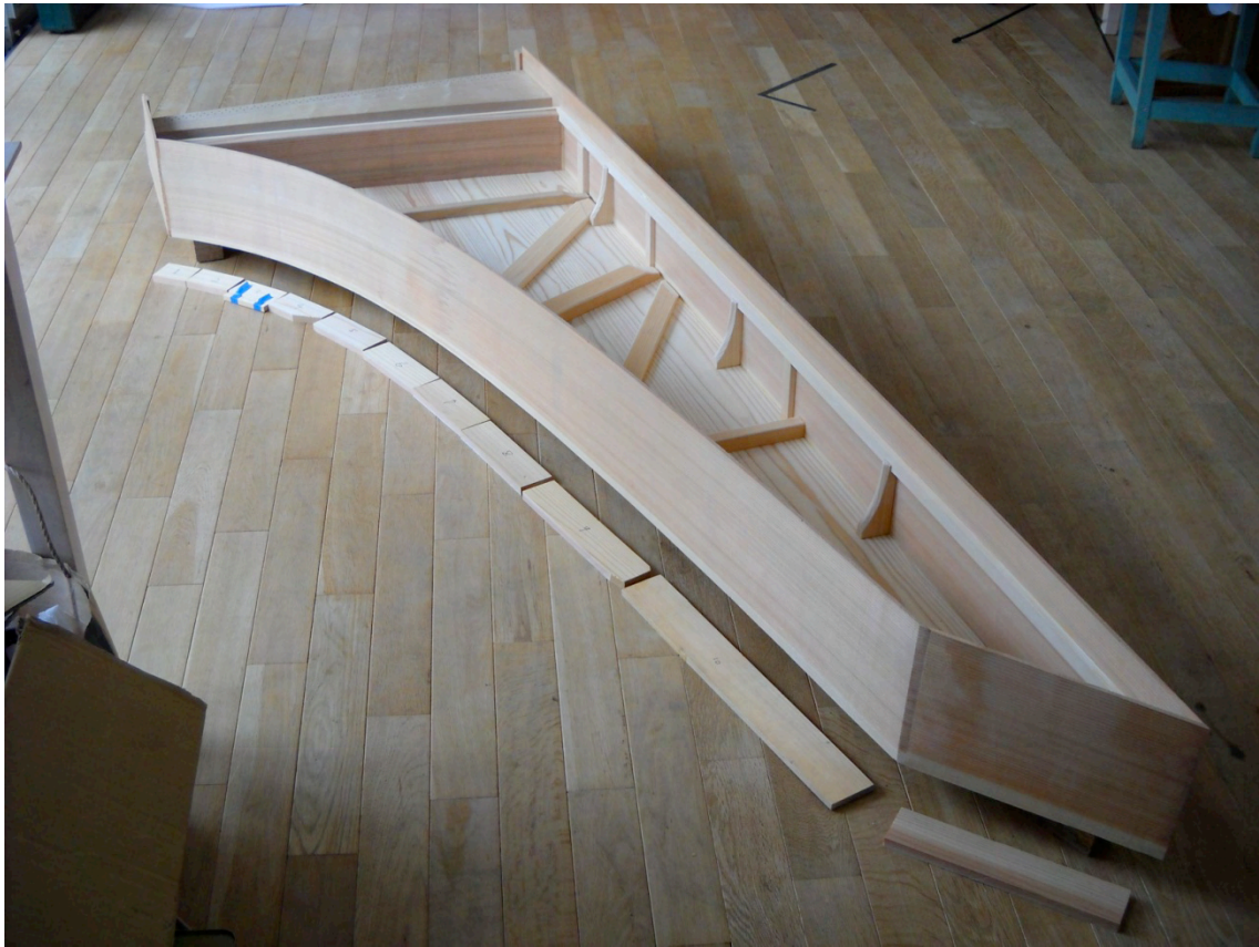
The wooden pieces for cramping the sound board is prepared and numbered.
