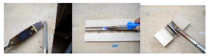
Burn the mortise using a solder iron with a tip for this use. You can easily make this tip by your self.
