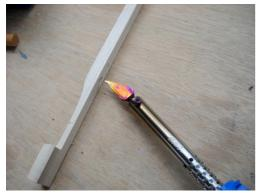
. This picture shows that the key is cut apart but you can burn the hole before the keys are cut apart. It is also important to burn the underside of the keys where the balance washers will touch the keys. I use cow skin for balance washers. Take care you will not burn too much you need to check often with your balance pin. Especially the top of the mortise is close to the solder iron, so the
