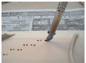
After the jack guide is glued beneath the sound board, you can drill two holes for each jack hole from under side. Then you can burn using the solder iron shaped above. The tip of this solder iron is designed for making balance pin mortises in burning method which will be shown bellow.
