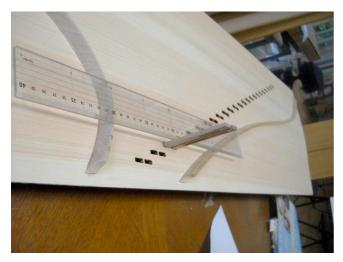
You can find where shall come the string to the right bridge. Especially you cannot get the positions of bridge pins from the drawing at the treble area where the jacks are closer to the right bridge. On the other hand on the left bridge the holes are drilled and burnt when you will string the instrument.
