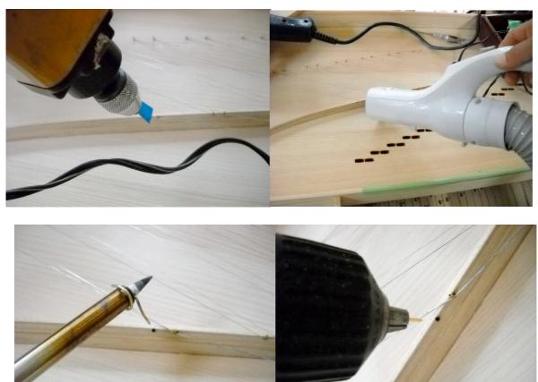
A bridge is chucked to the drill and it can be pushed in while turning.
